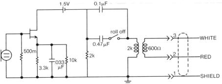
Positive (inward) acoustic pressure at diaphragm produces positive voltage at Pin #2.
